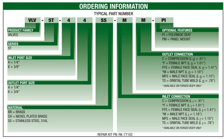
3 PORT, 4 PORT AND CUSTOM CONFIGURATIONS ARE AVAILABLE ON REQUEST. AVAILABLE WITH PNEUMATIC OPERATOR, SEE HPST-4 SERIES.
