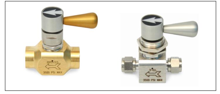
GasFlo Products QSL Series Valves provide quarter turn, positive shut off for critical gas/fluid systems. The lever handle design allows for visual open/closed indication and guick acting cycling. This springless diaphragm valve offers superior leak integrity for Specialty Gas, Chemical, Instrumentation, Semiconductor, Medical and general purpose applications with pressure ranges from vacuum to 3500 psig.
