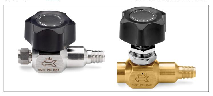
GasFlo Products LL Series Valves are manufactured with an extended inlet leg to allow handle clearance from mating equipment without the need for additional bushings. This economical springless, diaphragm design makes for the perfect regulator outlet valve, providing a positive shut off and smooth operation for pressure ranges from vacuum to 3500 psig.
