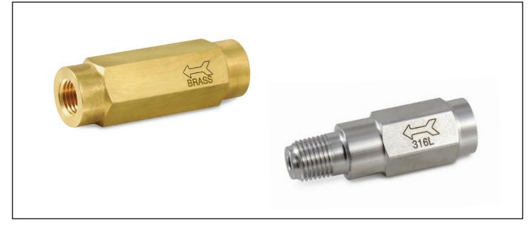
GasFlo Products CV-BS Series Check Valves prevent the reverse flow of gas/fluids and protects regulators, cylinder valves, purge assemblies and manifold systems. Manufactured from bar stock this poppet and spring design with an O-ring at the valve seat ensures positive shut off and guick acting response.
